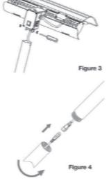
Pull gently on the cable at the bottom of the base to keep it taut. Fix the cable to the base with the cable clamp and (2) M4 screws.
